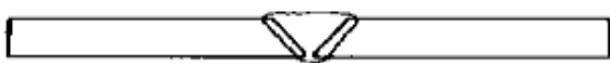
QW-463.1(b) PLATES — 3/4 IN. AND OVER THICKNESS AND ALTERNATE FROM 3/8 IN. BUT LESS THAN 3/4 IN. THICKNESS PROCEDURE QUALIFICATION
